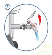
Pull up the water tap to let the sewage flow out 打开水龙头让污水流出
